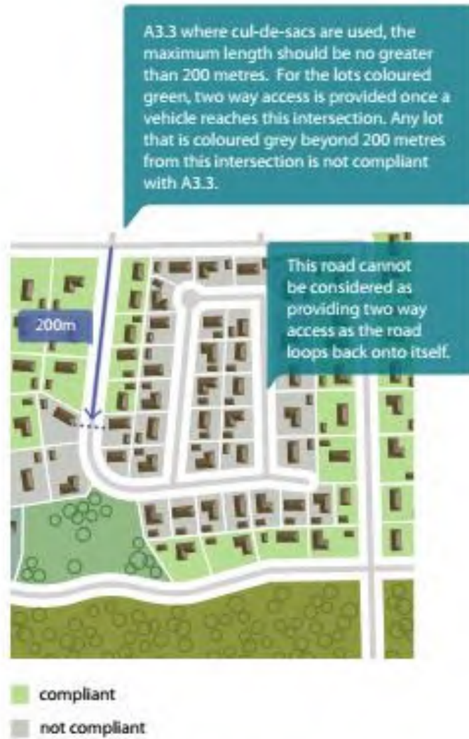
Figure 21: Example of compliant and non-compliant two-way
